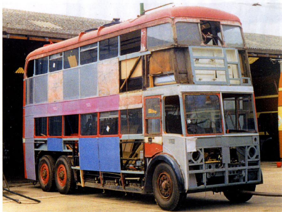
A progress picture taken during the restoration of 541. At this time a few windows and panels still remain to be replaced to complete the external restoration, before Brian turns his attention to the interior. (B Maguire)
