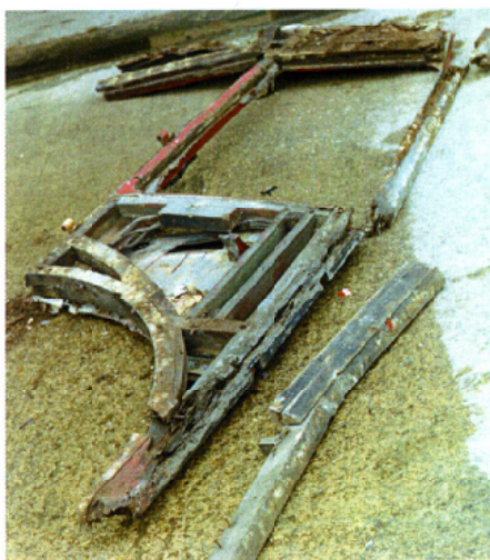
During the restoration, Brian Maguire's carpentry skills were sorely needed, as can be seen in this view of the rotten front offside of the driver's cab, after dismantling.
