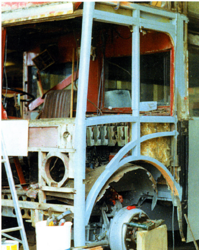
This picture illustrates the extensive nature of much of the restoration of 541. A major rebuild of the front nearside cab structure shows the intricate shaping and joinery required in the restoration of a wooden-framed vehicle. (B Maguire)
